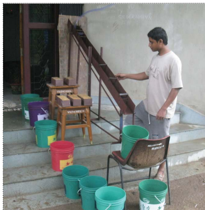
Figure 2. Hydraulic flume used to measure detachment rates from root permeated topsoil samples.
