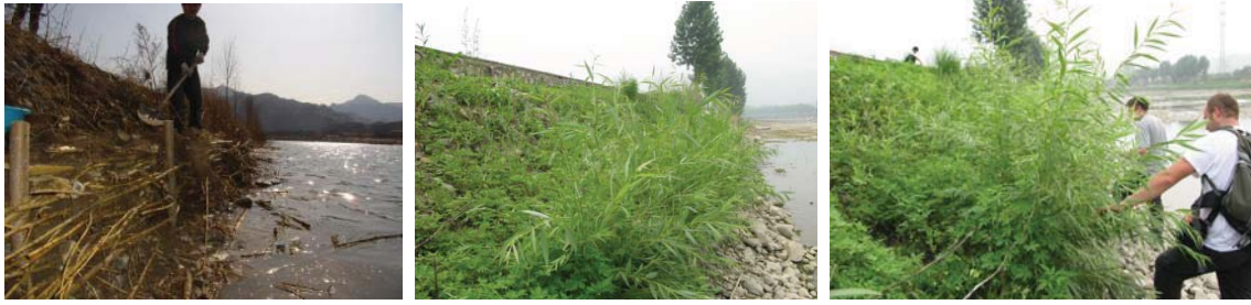
Figure 4. Experimental area by using wattle fence: the day of planting (left), 3 months after (middle) and 5.5 months after (right)
