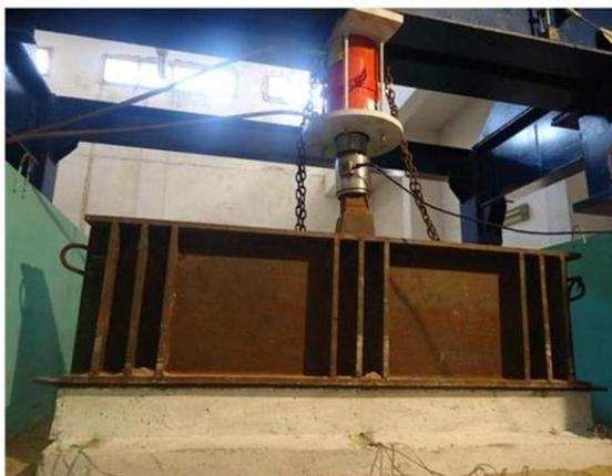
Figure (2) Sample Loading and Strain Gauges Arrangement
