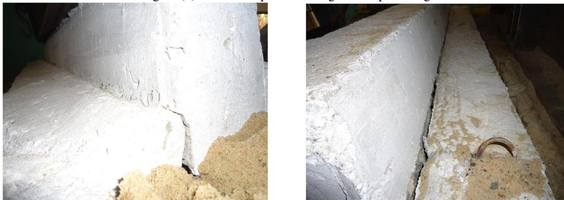
Figure (10) Failure Shape of Folded Strip Footing
