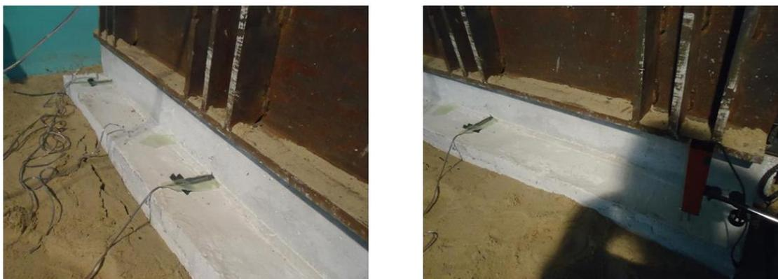
Figure (3) Measuring of Soil Settlement
