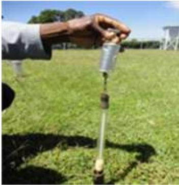
Figure 1: Symons-pattern earth thermometer  $\geq 30$  cm
