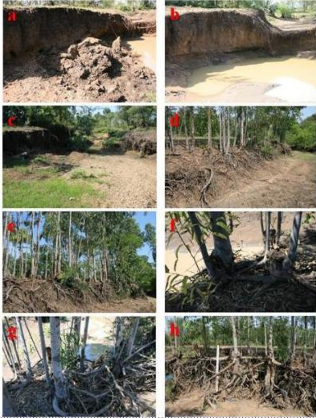
Figure 1. Field survey of Eucalyptus root system and its performance in blocking gully erosion development at Kokal village in Kisumu, western Kenya. Slumping of gully walls occur in the absence of Eucalyptus roots (a, b, c). Eucalyptus root system hold large soil mass preventing slumping of gully walls (c, d, e). Eucalyptus roots fused forming intimate mass of root system (f, g). Neighboring Eucalyptus supported adjacent tree whose roots were freed of soil by water erosion (h).
